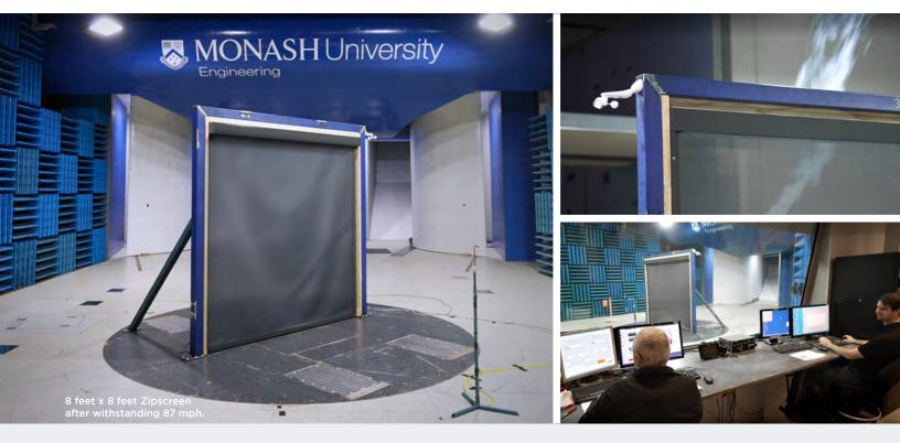
\*The Zipscreen shade used X-Weave 5% fabric and was side fixed to a timber substrate secured with 12G fasteners. Inner rails were secured with 8G fasteners as per the Zipscreen Installation Manual guidelines. Each wind speed test was held for a minimum of 60 seconds. 'Maximum achievable wind speed' refers to the limitations of the testing facility, and not the Zipscreen system.
